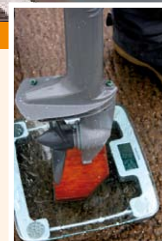
Weighing the engines to assess their fuel consumption
