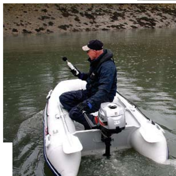
Bob checks the sound meter display having just taken a reading
